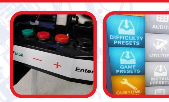
Use buttons inside coin door to access & navigate Test Menu.
